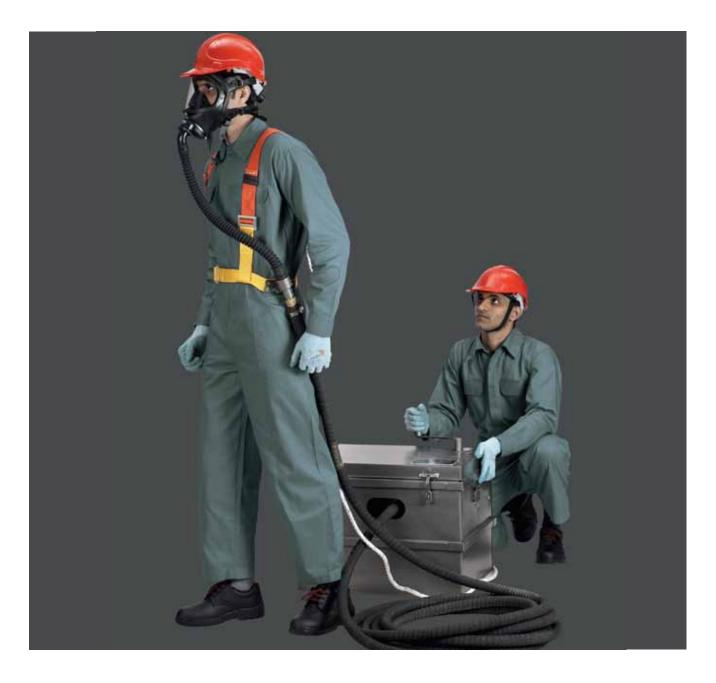
The JLD FRESH AIR HOSE APPARATUS consists of an ISI marked PROTECT 2000 Full Face Mask connected to a corrugated tube ending in a manifold mounted on a harness belt worn around the waist. The manifold is connected to a 15 meters long 20mm I.D. canvas covered wireembedded rubber hose. The other end of the hose is connected to the hand operated blower.
